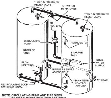
NOTE: CIRCULATING PUMP AND PIPE SIZES TO BE SELECTED FROM THE CER-TEMP 80 DIAGRAM FOR THE MODEL HEATER TO BE INSTALLED.
